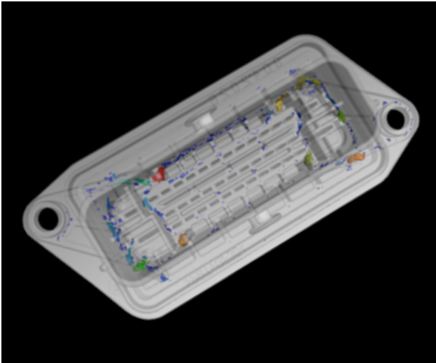
CT scan of a Plastic Connector
